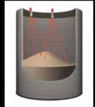
Adding an additional scanner in a wide bin provides more coverage of the material surface, ensuring greater accuracy!
