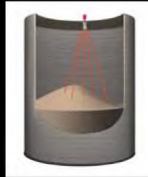
A single scanner measures in a 70° beam angle that does not cover the entire surface area.
