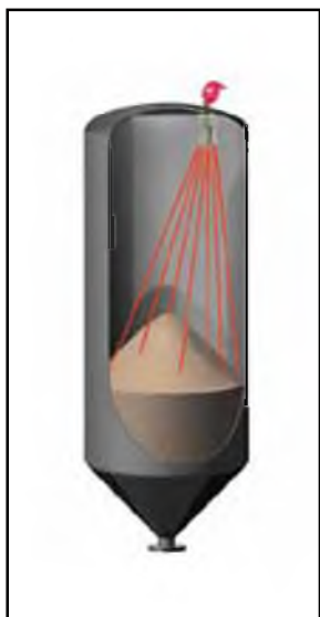
S model employs 30° beam angle for narrow bins.
