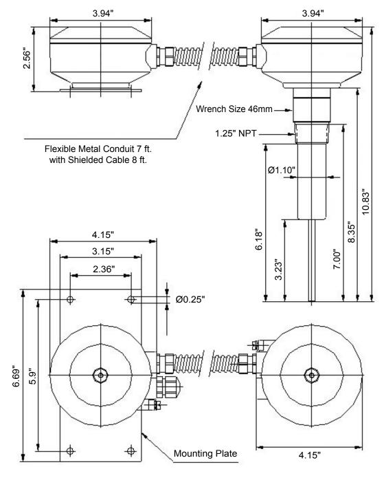
Assembling of probe, enclosure and electronics must be done according the following sketch.
